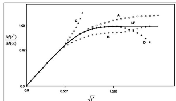
Figure 3. Schematic curves representing four categories of recorded non-Fickian weight-gain sorption
