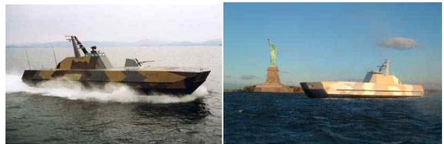
**Fig. 1. Skjold class patrol boat built with FRP sandwich**
