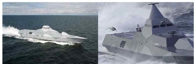
**Fig. 2. Visby corvette having hybrid carbon and glass fiber polymer laminate**
