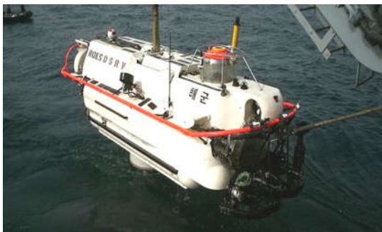
Fig. 1. Deep Submergence Rescue Vehicle(DSRV)
