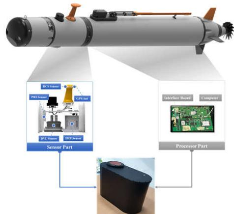
Fig. 2. Design concept of NTS(Navigation Test System)
